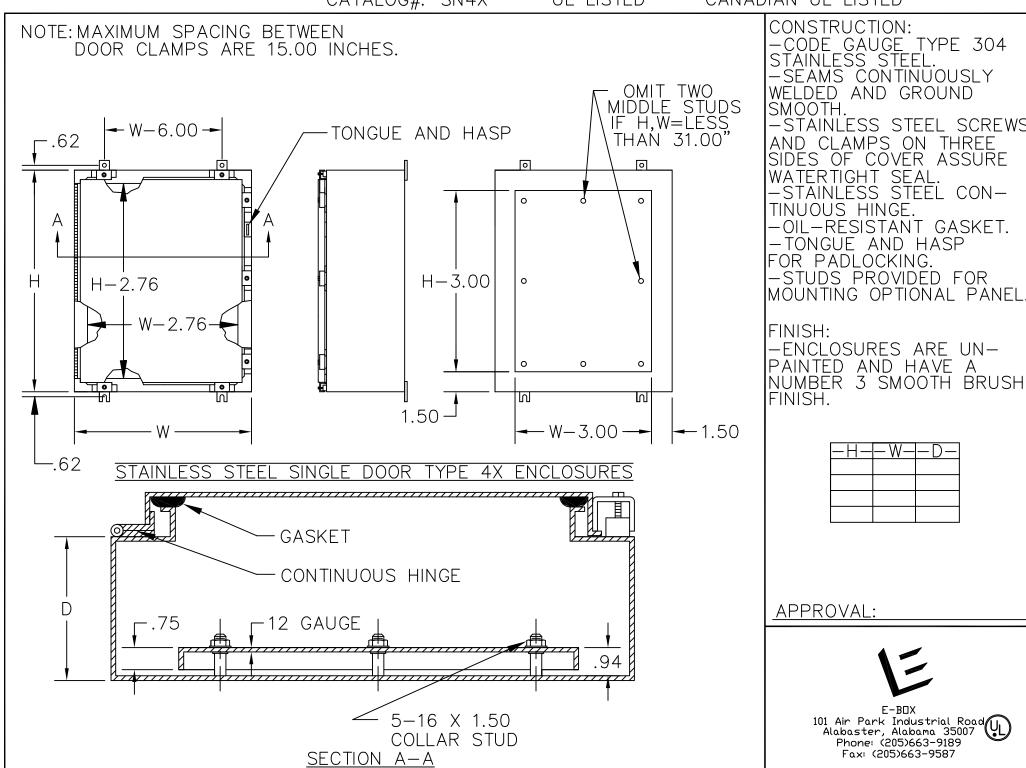
CONSTRUCTION: -CODE GAUGE TYPE 304 STAINLESS STEEL.
