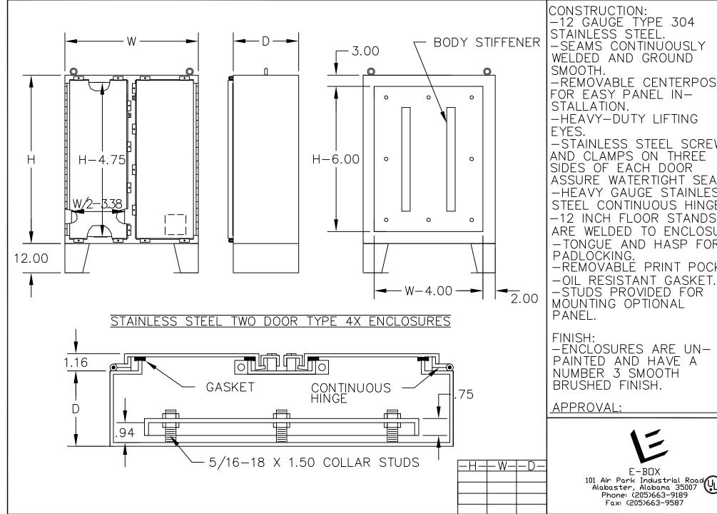
CONSTRUCTION: -12 GAUGE TYPE 304 STAINLESS STEEL. -SEAMS CONTINUOUSLY WELDED AND GROUND SMOOTH. -REMOVABLE CENTERPOST FOR EASY PANEL IN-STALLATION. -HEAVY-DUTY LIFTING EYES. -STAINLESS STEEL SCREWS AND CLAMPS ON THREE SIDES OF EACH DOOR ASSURE WATERTIGHT SEAL. -HEAVY GAUGE STAINLESS CONTINUOUS HINGE. 2 INCH FLOOR STANDS ARE WELDED TO ENCLOSURE. -TONGUE AND HASP FOR PADLOCKING. -REMOVABLE PRINT POCKET
