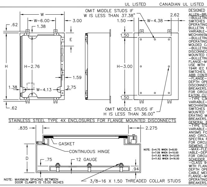
DESIGNED TO HOUSE THE FOLLOWING: CONSTRUCTION: ALLEN-BRADLEY -BULLETIN 1494V DISCONNECT SWITCHES WITH FLANGE-MOUNTED OPERATING MECHANISMS AND BULLETIN 1494V FLANGE-MOUNTED VARIABLE-DEPTH OPERATING MECHANISMS FOR CIRCUIT BREAKERS. -BULLETIN 140U FLEXIBLE CABLE OPERATING MECHANISMS FOR 140U MOLDED CASSE CIRCUIT BREAKERS -BULLETIN 1494C CABLE-OPERATED DISCONNECT SWITCHES WITH FLANGE-MOUNTED HANDLES. -BULLETIN 194RC CABLE-OPERATED FLANGE-MOUNTED HANDLES FOR USE WITH THE NFPA 79 COMPLIANT
