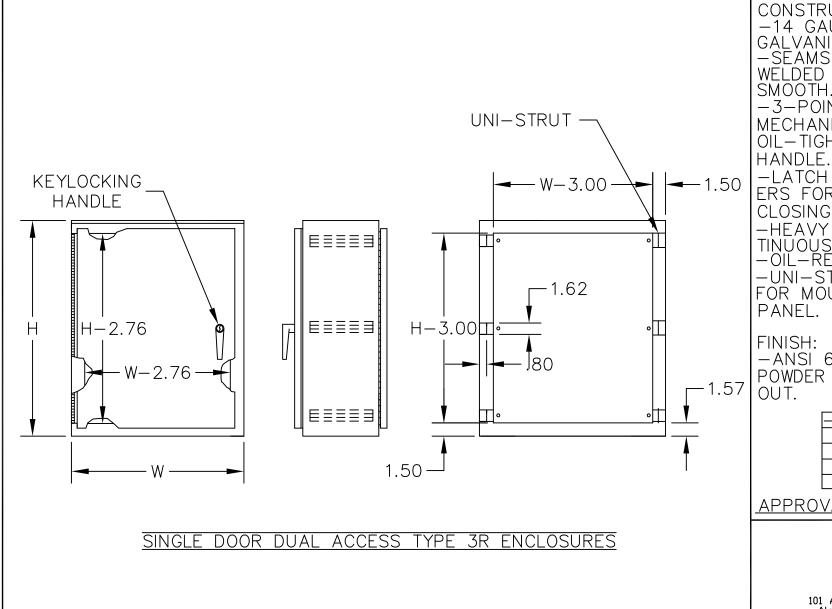
CONSTRUCTION: -14 GAUGE PAINT GRIP GALVANIZED STEEL -SEAMS CONTINUOUSLY WELDED AND GROUND SMOOTH. -3-POINT LATCHING MECHANISM OPERATED BY OIL-TIGHT KEYLOCKING
